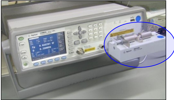
Fig.4 Measurement Equipment: LCRmeter E4980A (Keysight Technologies)
