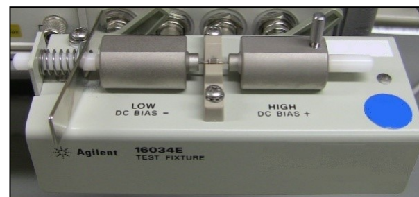
Fig.5 Measurement jig: Test fixture16034E/G (Keysight Technologies)
