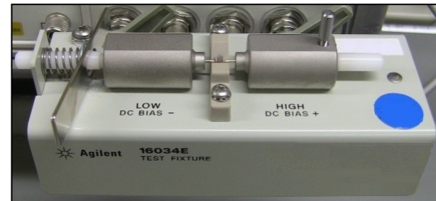
Fig.5 Measurement jig: Test fixture16034E/G (Keysight Technologies)
